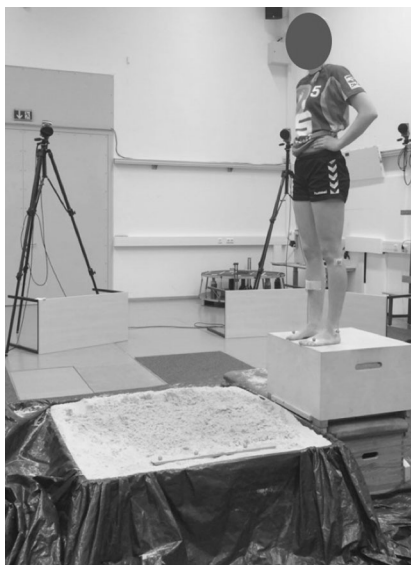
Fig. 1 ▲ Laboratory situation when measuring drop and countermovement jumps on sand and rigid surfaces. The figure shows a subject prior to performing a drop jump into the sandbox. For countermovement jumps, the drop-box was removed and athletes performed directly within the sandbox from sand level. The jumps on the rigid surface were performed on the floor directly behind the sandbox
